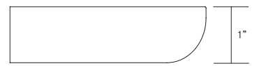
Edge Detail # 46 1" MDF core, specified melamine face and counterbalance. The edge is clear finish as standard.
